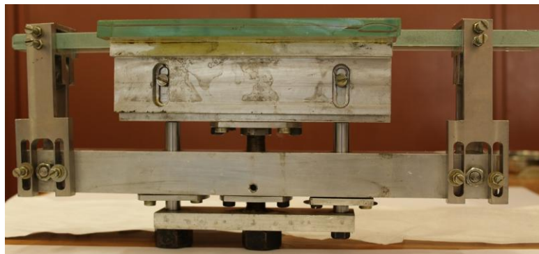
Figure 3: Bender with Glass Strip in Stress Condition
