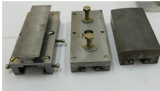
Figure 7: Dovetail Guide and Tool for Grinding
